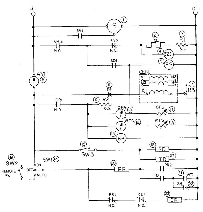
10-15 KW WPDS GENERATOR WITH AUXILIARY CHARGING WINDING AND STARTER DISCONNECTED BY CENTRIFUGAL SPEED SWITCH DRAWING NO. 13743
