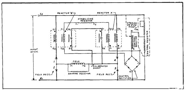
Fig. 4.G - Typical Magneciter Circuit
