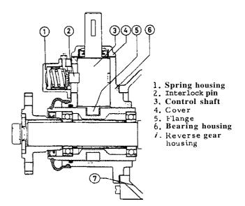
Fig. 3. Rear section of reverse gear
