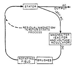
Fig. 4.A — Schematic, Alternator and Exciter
