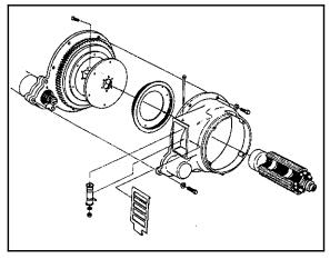
Fig. 4.N - Removing Rotor
