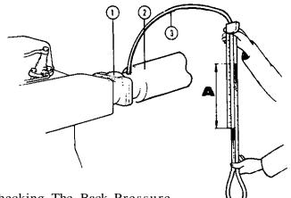
Checking The Back Pressure 1. Exhaust pipe flange
