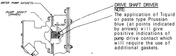
If the proper clearance is not maintained, the sea water pump shaft will force the fuel pump drive hub against its bushing. The bushing will seize to the drive hub and rotate in its housing. Bushing wear and loss of oil pressure will result.
