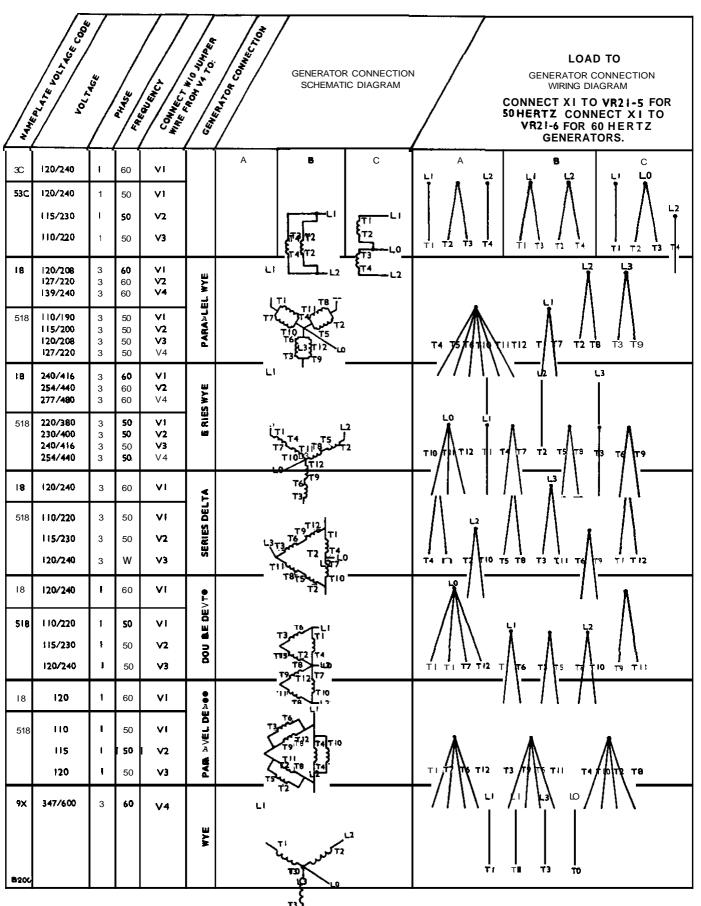
FIGURE 6. GENERATOR WIRING AND RECONNECTION DIAGRAMS
