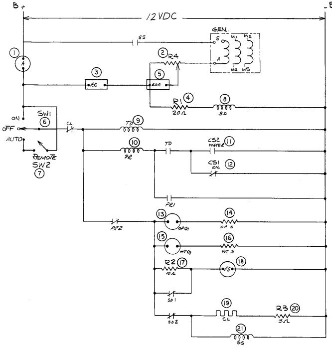
10-15 KW WPD GENERATOR WITH AUXILIARY CHARGING AND CRANKING WINDINGS **DRAWING NO. 12970**
