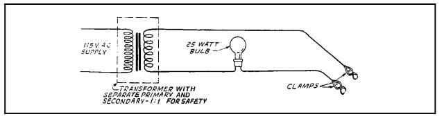
Fig. 4.K — 115V Continuity Test Lamp (Use for testing Magneciter)
