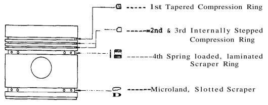
Piston Ring Arrangement Shown Four-107 Engines Rated up to 3000 RM RING SET, PART NUMBER 12906
