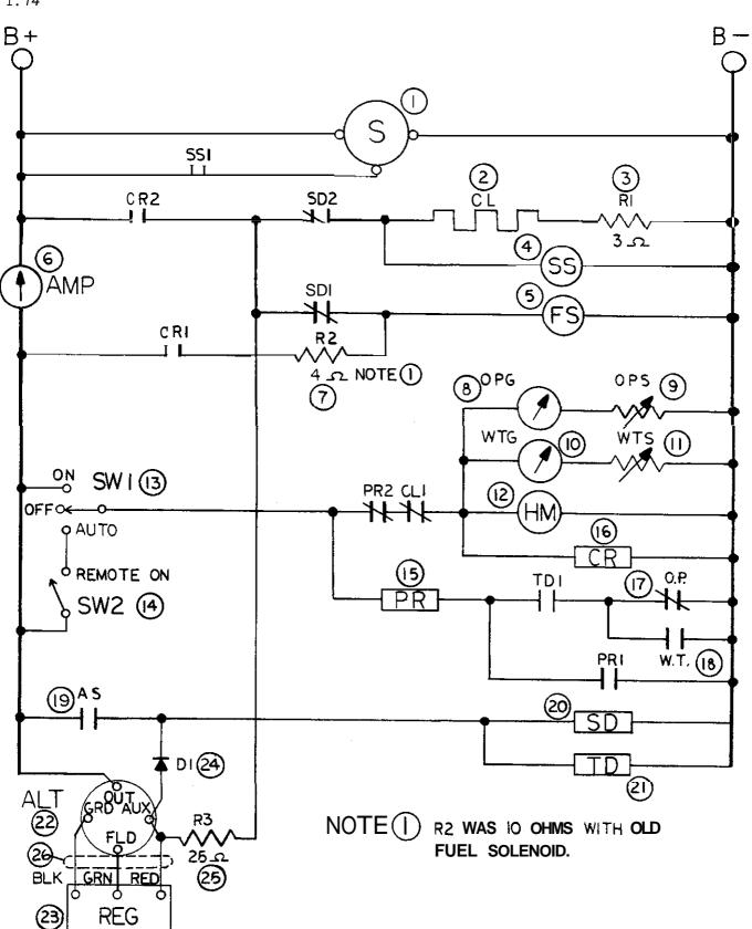
10-15 KW WPDS GENERATOR WITH STARTER DISCONNECTED BY AIR SWITCH **OR ALTERNATOR OUTPUT** DRAWING NO. 12868 C
