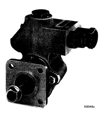
TYPE: • Fixed Displacement Piston Type ROTATION: • Clockwise or Counter-Clockwise SPEED: • 600 RPM to 3600 RPM\* UNLOADING VALVE: • Integral and Pressure Adjustable PRESSURE ADJUSTMENT RANGE: • 1500-3000 PSI NORMAL PRESSURE CUT-OUT: • 3000 PSI NORMAL PRESSURE CUT-IN: • 2500 PSI SELF PRIMING AND SELF BLEEDING MAXIMUM SUCTION HEAD: • 3 Ft. HOUSING: • Cast Aluminum WEIGHT: • 5 • 1/2 lbs. DRIVE TORQUE: • 9 in. lbs. @ O-PSI 28 in. lbs. @ 3000 PSI
