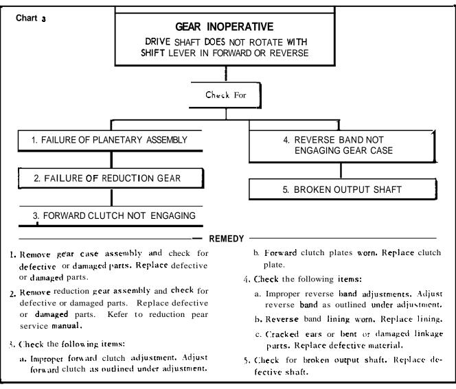
NOTE: Disassembly need be carried out only as far as is necessary to correct those difficulties which interfere with proper marine gear operation.
