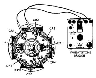
FIGURE 15. TESTING EXCITER ARMATURE
