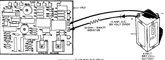
FIGURE 8. FLASHING THE FIELD
