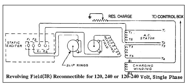
Fig. 4.Q-Internal Generating Diagram.
