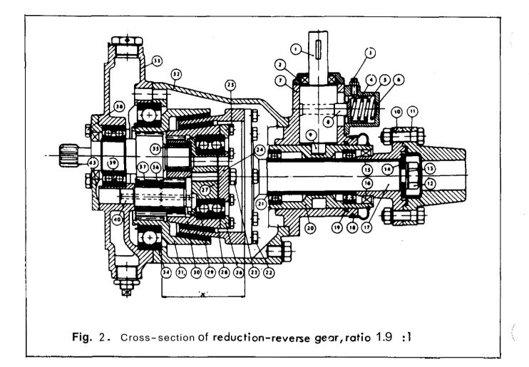
sure is applied to the shaft journal for the bearing (35). Take care to ensure that the needle bearing (35) is not damaged. Protect the bearing from dirt and place it so that it will take up the same position again when being fitted.
