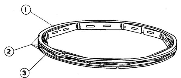
The gaps of the remaining rings should be staggered alternately along the piston pin axis. Liberally lubricate the rings in their grooves and see that they can move freely in their locations. this does not apply to the laminated type in the fourth groove, which if correctly fitted **should** not move freely due to the outward pressure of the top and bottom segments on the ring groove walls. When ail the rings have been fitted, they should
