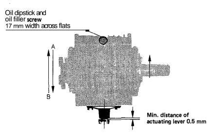
The position of the cover plate underneath the actuating lever is factory-adjusted to ensure equal lever travel from neutral position to A and B.
