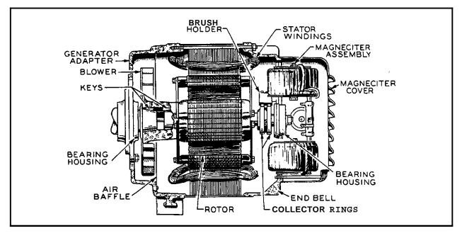
Fig. 4.B - Revolving Field Generator Cross Section
