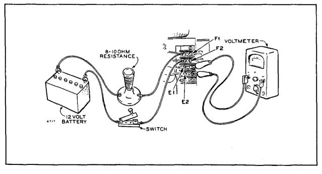
Fig. 4.I - Flashing the Field See Sect. 4.3.1.1.
