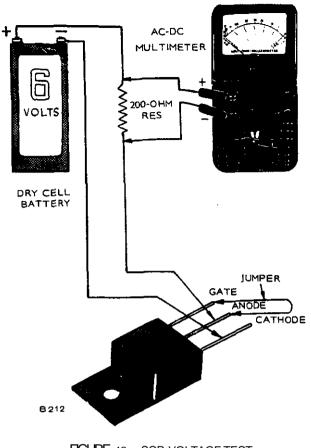
FGURE 13. SCR VOLTAGE TEST
