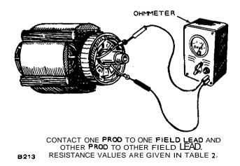
FIGURE 17. TESTING ROTOR FOR AN OPEN CIRCUIT
