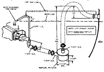
WATER LIFT EXHAUST SYSTEM WITH "HYDRO-HUSH" MUFFLER If there are more components to be rigidly connected to each other than will weigh 8 pounds, then a flexible exhaust section must be installed between the manifold outlet and the exhaust system.
