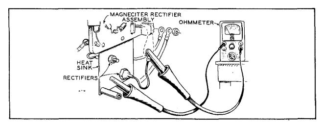
Fig. 4.M — Testing Field Rectifier
