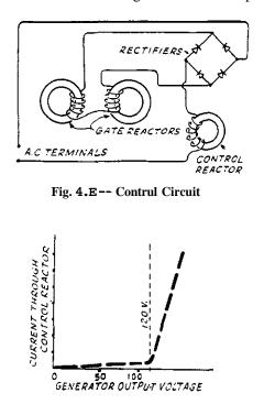
Fig. 4.F - Control Reactor Characteristics
