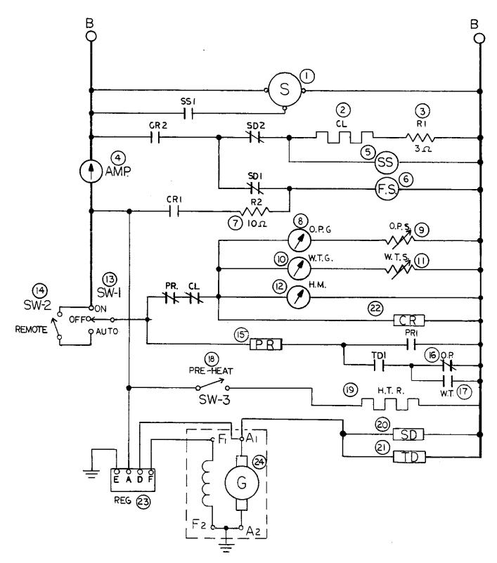
10-15 KW WPDS GENERATOR WITH STARTER DISCONNECTED BY D.C. BATTERY CHARGING GENERATOR DRAWING NO. 13742
