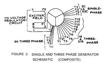
connected to the output terminals of the voltage regulator. Leads 1 and 2 are connected to the stator windings and provide reference voltage and input power to the voltage regulator. These five leads are connected at the factory.
