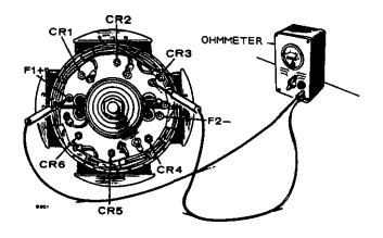
FIGURE 9. TESTING ROTATING RECTIFIERS
